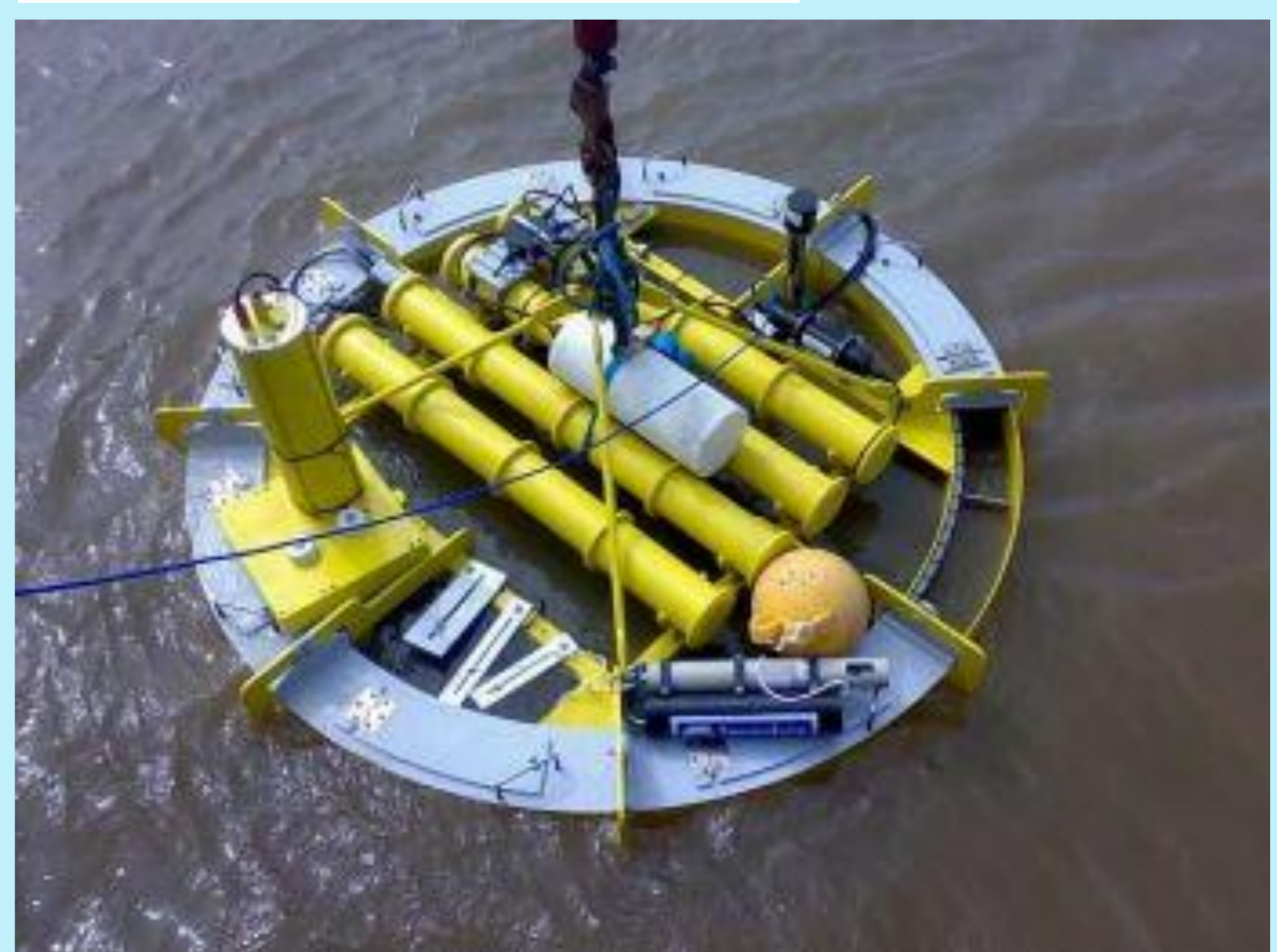
Figure 5: In-situ annular flume from Partrac Ltd
